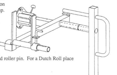
When rolled, remove hose and handle at the same time, lay hose flat and remove handle.
