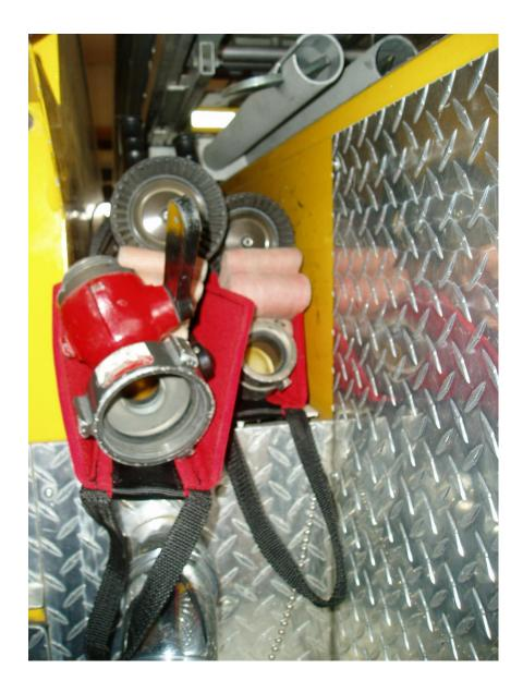
If your hose compartment has no cover, use a small strap to secure the hose packs in the compartment.
