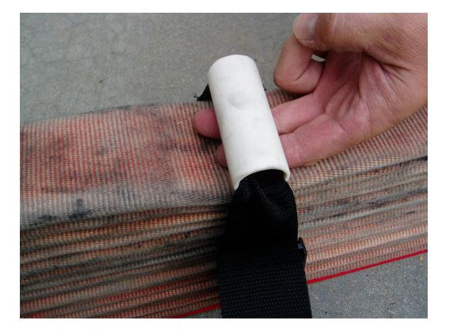
13. Finally, velcro the tails of the straps to the opposite side from the buckles to keep them out of the way.
