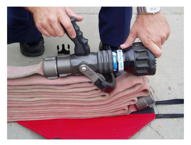
After the fourth fold, use the same method to determine the nozzle placement so that the strap passes just forward of the pistol grip.
