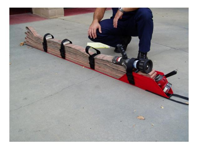
The only difference in the second pack is that the *female coupling*, instead of the gated wye will be initially placed at the front of the pack to begin the load and then flakes will be stacked up behind it.
