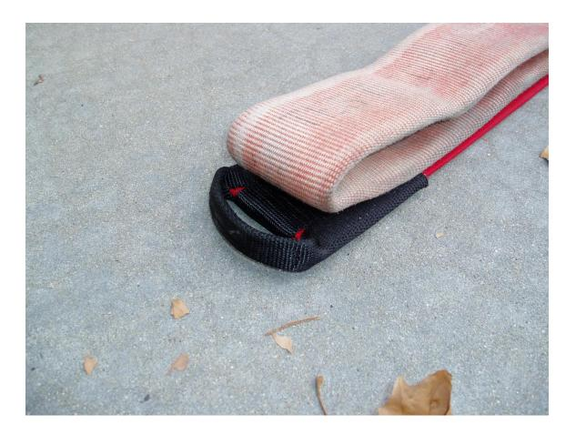
5. Make the second fold right up next to the wye. Continue making flakes in this manner, filling up the pack. It is important that the flakes on the front end (close to the wye) have the folds stacked directly on top of each other.
